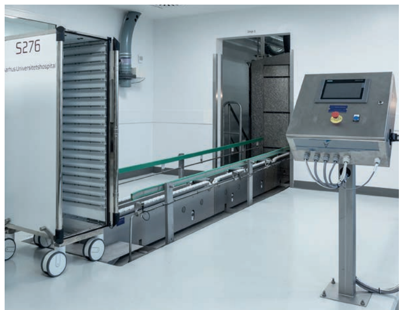
Automatic cleaning system at Aarhus University Hospital for case carts and plastic boxes.
